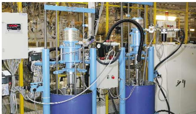
Double ram system with automatic switchover
